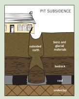
Pit subsidence forms a bell-shaped hole 6-8 feet deep and from 2-40 feet across and occurs when a shallow mine roof collapses.
