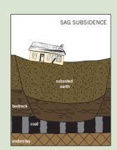
Sag subsidence, the most common type of mine subsidence, appears as a gentle depression in the ground and can spread over an area as large as several acres. Collapse of pillars supporting the mine roof is a typical cause.
