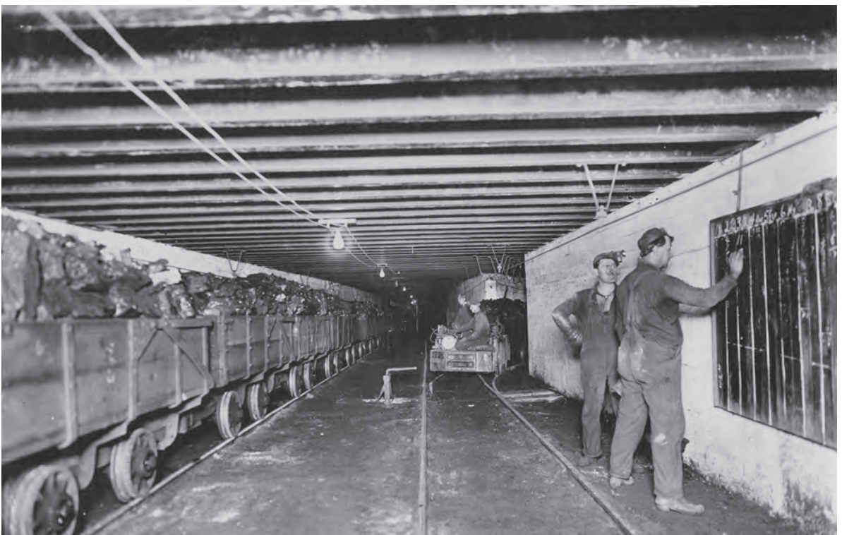
Top left: Mine workers hand loading a coal car. The man on the far right is most likely a driver waiting for the car to be filled. ISGS, circa 1920.
